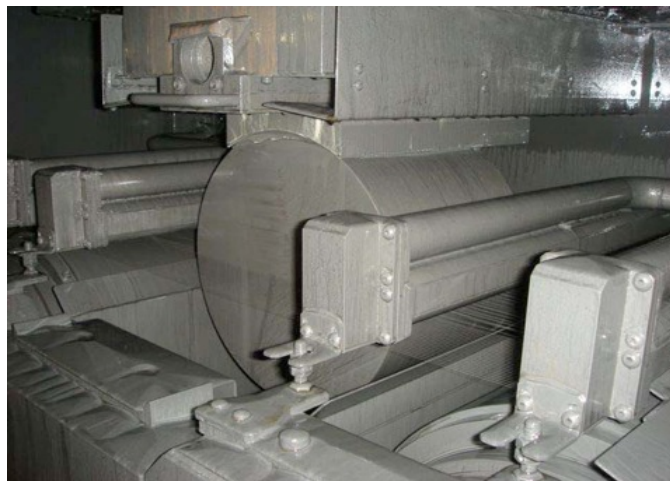
Figure 2: Large grain niobium sheet multi-wire saw technology
