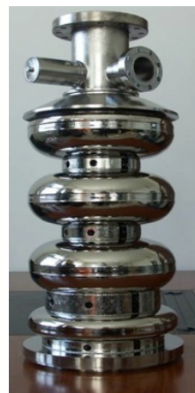
Figure 6: Large grain niobium sheet made by OTIC used to produce superconducting cavities at Beijing University and its performance
