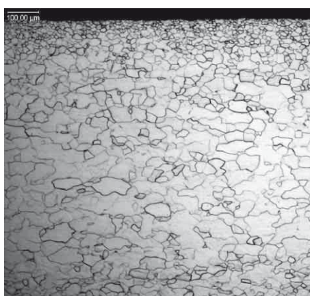
Figure 4: Typical Microstructure for Platinum Modified NRC76 Alloys
