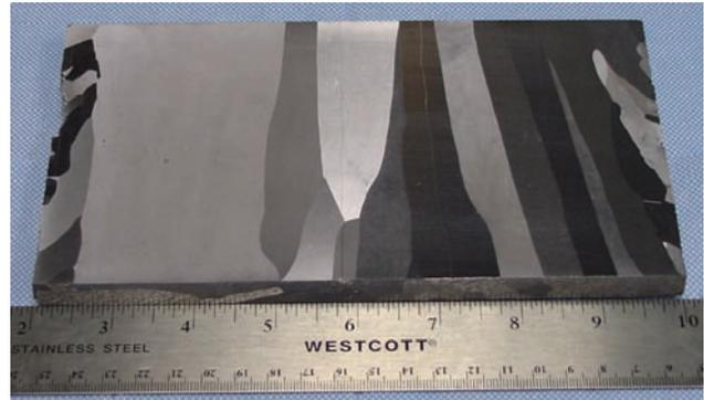
Figure 5: Ingot longitudinal section
