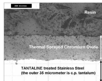
Figure 5: Cross-section of a Tantaline™ treated part subsequently thermally sprayed
