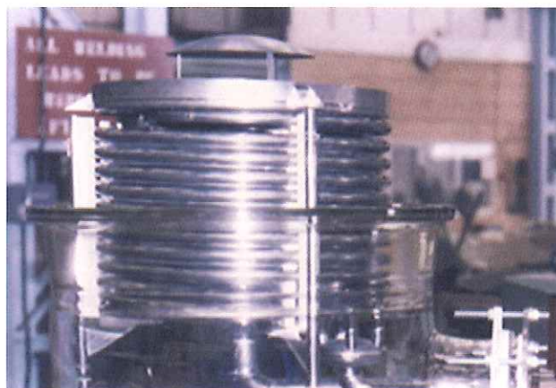
Fig 7: Multi-turn tantalum helix condenser assembly inside a glass vessel
