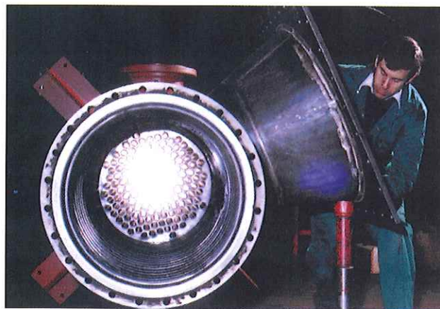
Fig. 4: Conical condenser at end of a tantalum shell and tube heat exchanger showing rigidising of the tantalum lining to withstand vacuum conditions.
